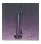
The sampling dipper or other sampling device must be of sanitary design, clean, in good repair, and of proper construction (i.e., free of pits, cracks and crevices) stored in the sampling instrument container, with an approved sanitizing solution of the proper strength. The sample dipper is used to aseptically transfer a sample of milk from the bulk tank or milk can to the sample container used to carry the sample to the official laboratory.
