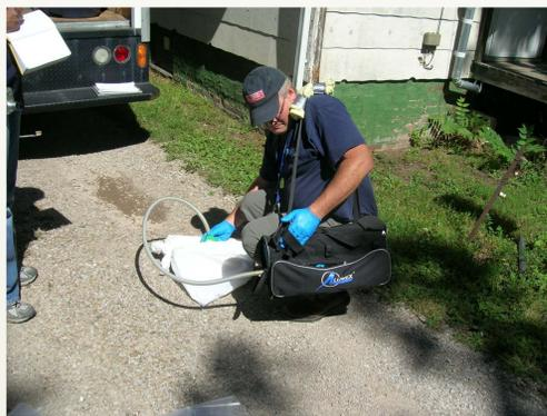
Contractor using Lumex mercury analyzer. Photo © to Aaron Martin
