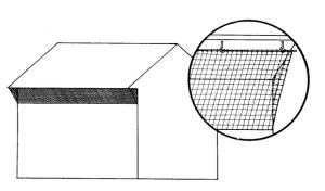
Figure 5. A net to prevent damage by woodpeckers. Image by Prevention and Control of Wildlife Damage (PCWD).
