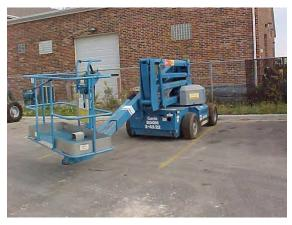
Figure 7. Bucket lifts can provide a safer and more efficient way to work in high areas. Photo by Stephen M. Vantassel.
