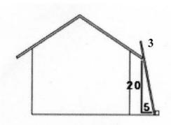
Figure 6. Diagram of the proper positioning of a ladder (note 20:5 = 4:1 ratio of rise to run). Image by NWCO Best Practices Guide.
