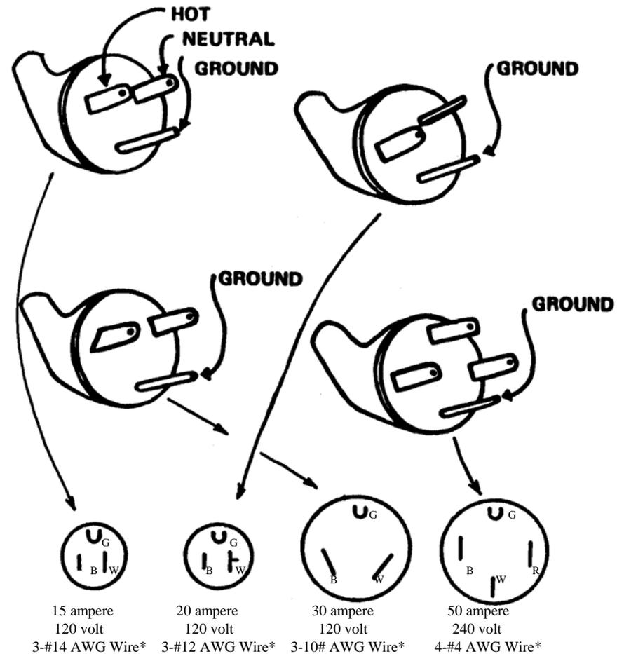
\* Recommended Cord Size. Use only cords manufactured for hard use. Never use a cord with only two conductors or one which does not have a ground pin on its plug. Cord length should be at least 20 feet and normally not more than 26 feet long. If longer cords are used they should be at least one wire gauge (AWG) larger. Extension cords are not recommended and if used may cause GFI circuit breakers to trip out.
