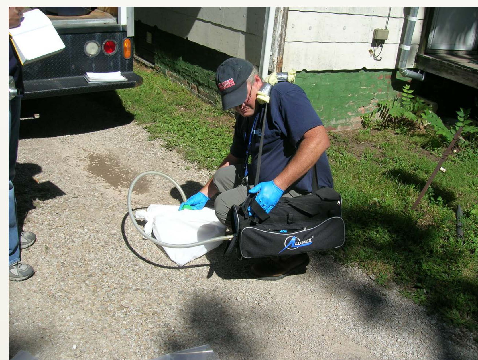
Contractor using Lumex mercury analyzer. Photo © to Aaron Martin
